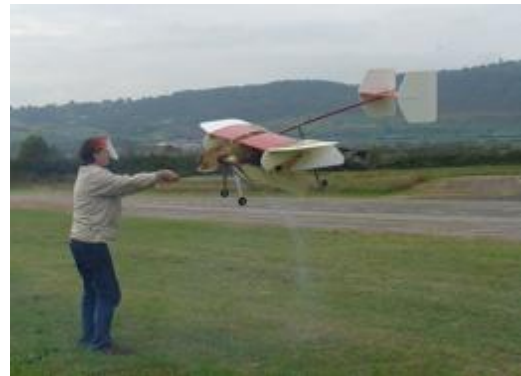
Fig. 5 Tethered VTOL hovering tests
