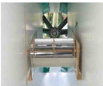
Fig 8 2-D wind tunnel tests in 2010 & 2012
