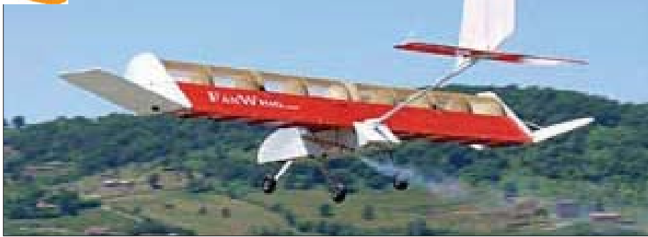
Above: The latest FanWing UAV demonstrator added winglets to the design.
